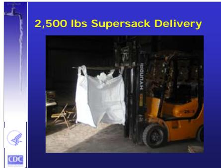
Supersacks are a 2,500-pound delivery package that is common in the bulk handling market, and sodium fluorosilicate is available for delivery in supersacks. They hold the equivalent of one pallet of bags. Supersacks have forklift loops for lifting and transporting. For facilities that use a lot of sodium fluorosilicate that can be designed with a large storage hopper, this can be a cost-effective means of handling the additive.
