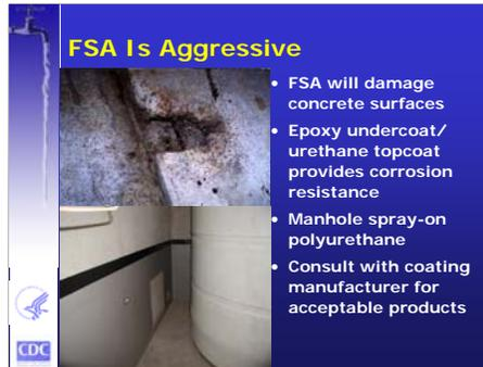
FSA will damage concrete surfaces. Along with the use of corrosion-resistant pipe materials, provide surface protection to the concrete where leaks could occur.
