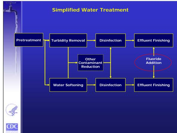
Here is a simplified schematic diagram of water treatment. The top line would be a conventional surface water treatment facility flow train, and the bottom one would be groundwater system that requires some processing of the extracted water. You will see that water fluoridation would be like corrosion control in that it would be done as part of effluent finishing as the water is delivered to the water system for distribution.
