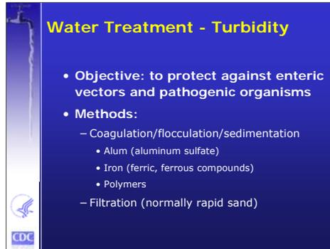
The slide features a dark blue background with a vertical gradient on the left side. At the top left, there is a small image of a water tap. The title 'Water Treatment - Turbidity' is written in yellow. The main content is a bulleted list in white text. At the bottom left, there is a small logo of an eagle and the text 'CDC'.
