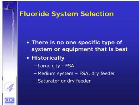
There is no one specific type of equipment that is used solely for one type of water system. All the fluoridation equipment, with the exception of a saturator, can be used on any system.
