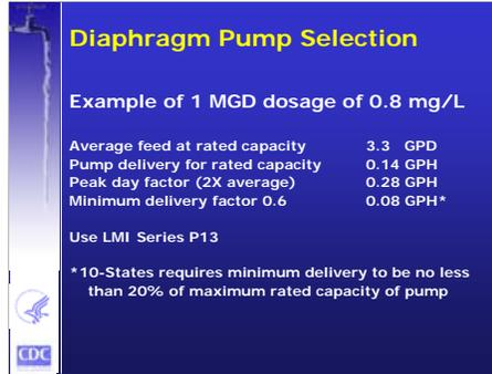
A blue slide titled "Diaphragm Pump Selection" with a CDC logo on the left. It provides an example of a 1 MGD dosage of 0.8 mg/L and lists pump specifications: Average feed at rated capacity (3.3 GPD), Pump delivery for rated capacity (0.14 GPH), Peak day factor (2X average) (0.28 GPH), and Minimum delivery factor 0.6 (0.08 GPH\*). It recommends using LMI Series P13 and includes a note that 10 states require minimum delivery to be no less than 20% of maximum rated capacity of pump.
