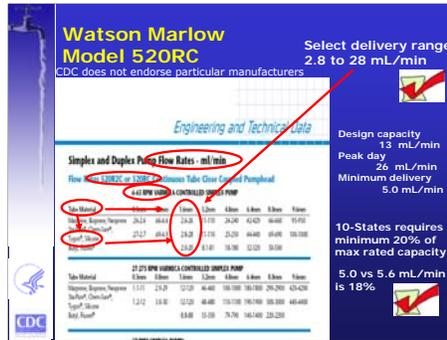
In this example, we have chosen a pump with a delivery pressure of up to 30 psi, having the delivery range from 2.8 to 28 mL/min to cover our range of 5.0 to 26 mL/min. We selected a tubing diameter to limit the delivery so that we will not over-dose the system. You can further increase or decrease the delivery of this pump by changing the tubing diameter.
