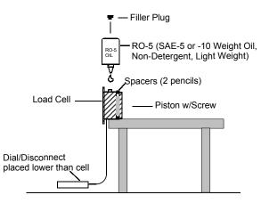
ADDING FLUID--STEP B: With the Load Cell higher than the dial and or disconnect, and the load cell plug facing skyward, remove the plug on the side of the cell. Pull the top plate apart just enough to slide a pencil (to be used as 5/16" spacer) under the edge of each side to create and even 5/16" gap. Take care not to exceed 5/16" to avoid damaging the internal diaphragm.
